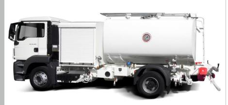
A 12,500L useable capacity rigid refueller mounted on a 6x4 chassis. The refueller is equipped with 1 x underwing and 1 x overwing hose, single meter and filter water separator or an optional filter monitor. Options include a weatherproof cabinet. The refueller conforms to latest European Standards EN12312-5 and JIG1 Issue 12 requirements.
